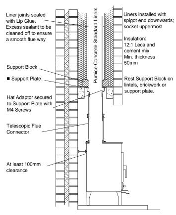
■ The Support Plate is designed to spread the weight of liners onto brickwork, reinforced concrete lintels or angle iron supports; it is not designed to support the weight of an entire chimney stack.
