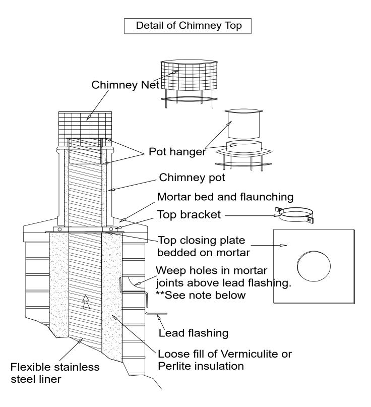
\*\* IMPORTANT Weep holes must not be placed facing into the prevailing wind
